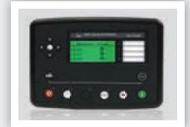
eliminates multiple analog gauges and switches for monitoring generator output (volts, amps and frequency for each output leg), battery voltage, coolant temperature, oil pressure, fuel level, engine speed and engine hours. In addition to accurate operating information, warning and safety shutdown messages are shown on the LCD display.
